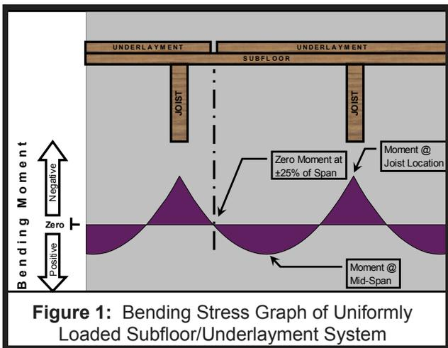
**Figure 1:** Bending Stress Graph of Uniformly Loaded Subfloor/Underlayment System
