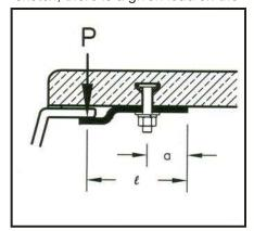
clip (referenced as "P"), but the load on the anchor is greater than that due to the leverage of the clip. The load on the anchor in this case would actually be  $(P \cdot \ell) \div a$ .
